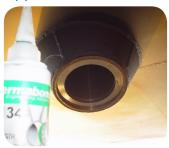
Adhesives are very good alternatives to welding or brazing. Gap filling and strong bonds in one step allows for relaxed tolerances of machined parts.
