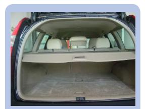
Application: Luggage Covers Bonding special automotive grade "Green (recyclable) PVC" around a roller. This is seen in the rear of many hatch / estate-type vehicles for covering luggage.
