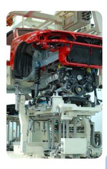
By replacing mechanical fasteners with adhesives, manufactured components are reduced in weight without sacrificing performance. Adhesives improve stress distribution and expand the choices of composites and dissimilar substrates throughout the vehicle.
