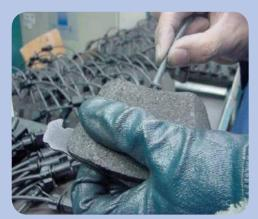
Application: Brake wear sensors Wear sensor wires are bonded into vehicle brake pads
