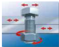
Vibration and loosening.
