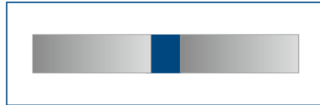
BUTT JOINT: A butt joint is formed by bonding two objects end to end.
