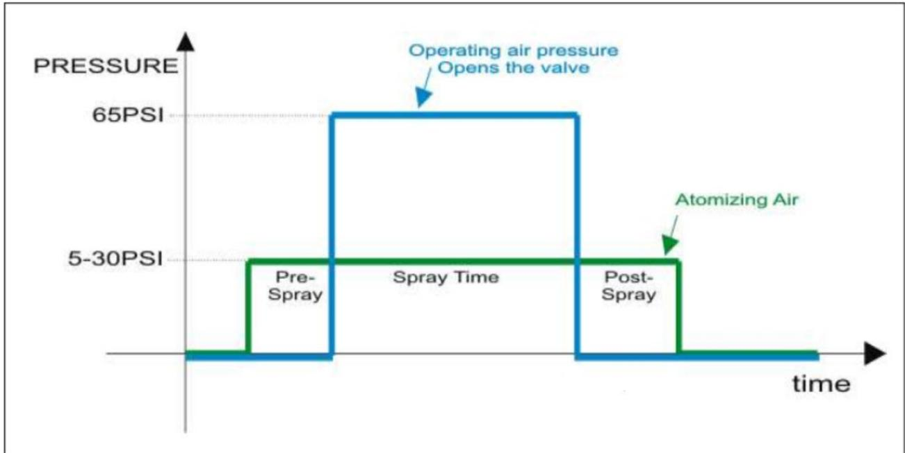
**FIG. 7: Timing Diagram**
