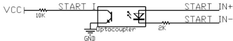
**FIG. 33: Example of I/O input port driving (pin #8)**
