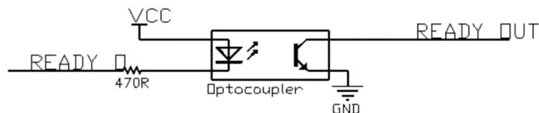
FIG. 30: Example of I/O output port driving
