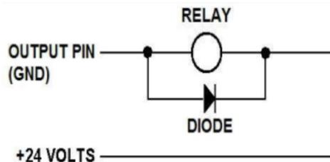
FIG. 31: Installation of Diode
