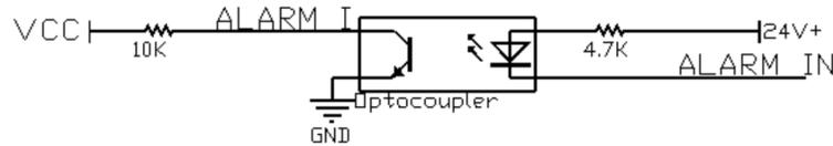
**FIG. 32: Example of I/O input port driving (pin #3, #4)**
