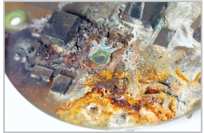
A PCB severely water damaged.
