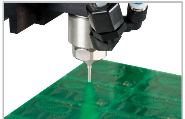
An automated Fisnar robot applying conformal coating.
