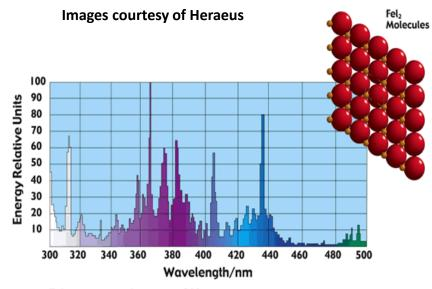
Enhances spectral output at 380 nm TYPICAL APPLICATION: UV curing of inks and varnishes responsive to 380 nm wavelength
