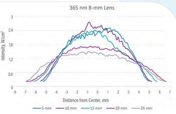
Note: Curing area data taken using Fuji UV Light Distribution Mapping System and normalized to ACCU-CAL<sup>™</sup> 50 LED Radiometer.
