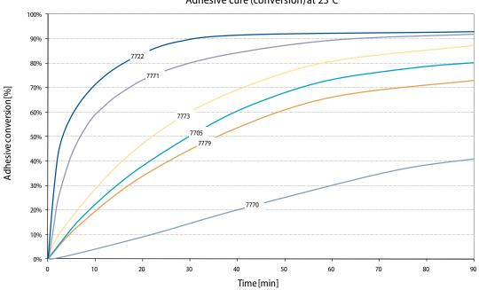
Depending on the parts size and shape handling strength is obtained at a fractional conversion of app 40-50%. Process strength (milling, sanding, painting) is reached at app 60-70%.
