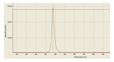
Figure 31. *BlueWave LED Flood* with VisiCure<sup>®</sup> Array – 405 nm Spectral Output
