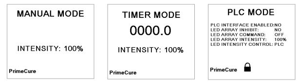
**NOTE:** If the BlueWave LED Flood System powers up in PLC Mode, you cannot change any settings via the front panel controls until you press the PLC Access Switch on the back panel.
