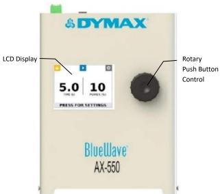
**Note:** The selected value will appear in blue color, when selected value requires modification press the rotary pushbutton, then, this value will turn yellow indicating it is ready to be modified. Turning the rotary pushbutton changes the value to be selected.
