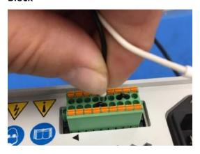
Figure 10. Insert Soft Wire or Pull Wire Out of Terminal Block
