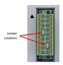
Figure 13. Example Connection for LED INHIBIT and MASTER INTERLOCK
