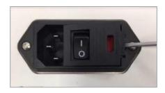
Figure 40. Lift Fuse Holder
